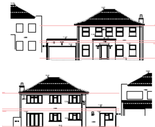
Figure 3 - Existing front and rear elevations
